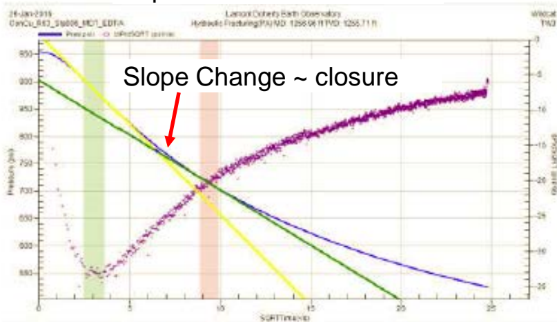
Figure 14: MDT-DP Microfrac 1,257 ft. cycle 1 pressure response, square root time and G-function analysis
